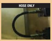
The LifeGuard<sup>™</sup> sleeve contained and effectively redirected fluid during 10,000 psi (68.9 MPa) burst tests while hoses without sleeving exploded, releasing a large amount of fluid in the immediate area.
