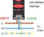
Parallel connection of ESP 415 M1, ESP 208 M1 or ESP 480 M1 to three phase star (4 wire and earth) supplies (fuses not shown for clarity)
